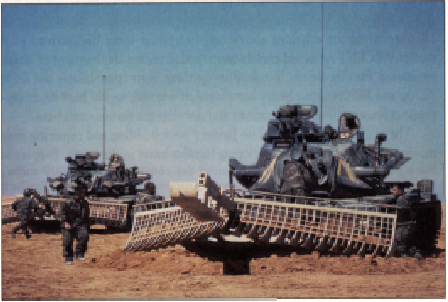
Soldiers of the 72d Engineer Company, 24th Infantry Division, test a mine clearing rake attached to an M-728 combat engineer vehicle.
