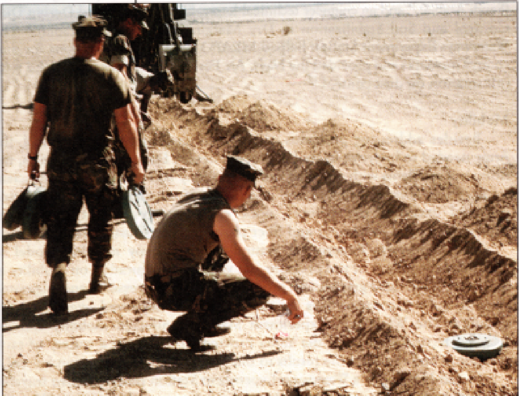
Marines place inert mines at Twentynine Palms, California, to test how well remote sensing techniques detect buried and surface mines.
