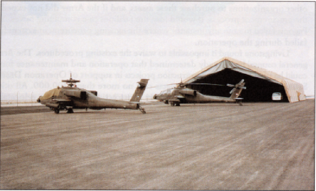
Clamshell buildings, manufactured in Santa Barbara, California, were used for aviation maintenance. Here, two AH-64 helicopters await maintenance outside a clamshell structure at King Fahd International Airport. Sand has eroded the blades from the Apache in the foreground costing $180,000 in repairs.
